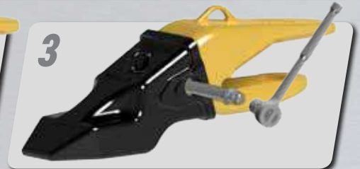
Insert Helical Pin & Rotate 180 degrees with Socket Wrench to Engage Lock
